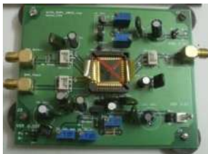
Test Board for Gm-C & Active RC Filters
